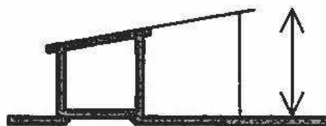
Figure 6 An enabling initial design of a core house as it does not constrain future extensions in relation to minimal height of the walls.
