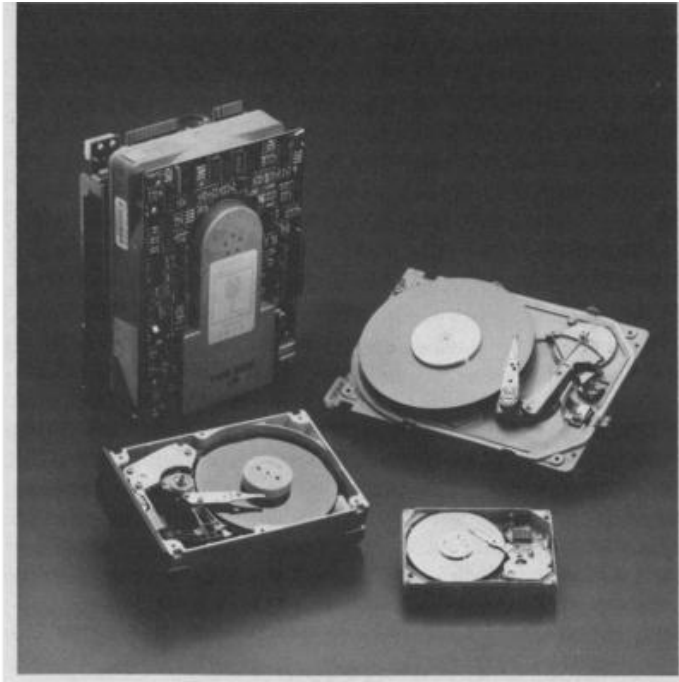
Modern Disk Drives • Shown, clockwise from upper left, are a 20 megabyte full-height 5.25-inch drive used in an early IBM AT personal computer; a 20 MB 5.25-inch drive that was half that height, to allow space for an additional floppy drive in the AT; a 2.5-inch drive (40 MB) used in notebook computers; and a 3.5-inch drive used in early portable and laptop computers. (Photograph, of disk drives in the author's possession, by Ed Malitsky, Boston, Mass.)
