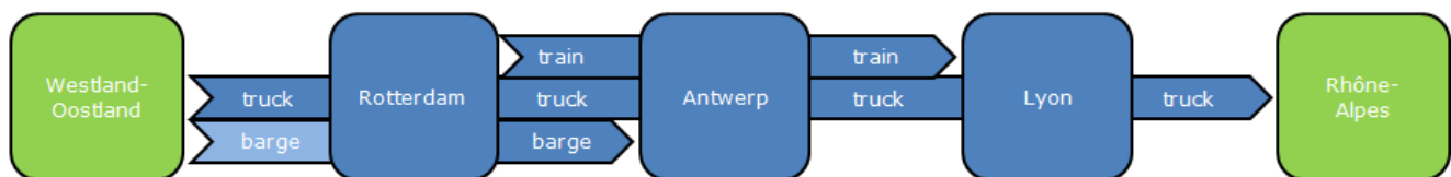
Figure 15: The hubs and modalities of a synchromodal corridor between the greenport and the Rhône-Alpes region.
