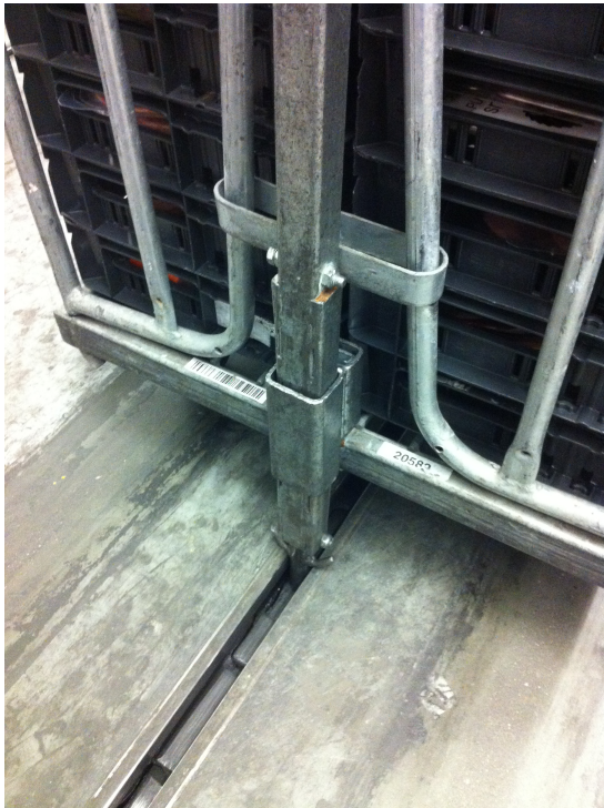
(a) System to couple and decouple carriers onto the chain.
