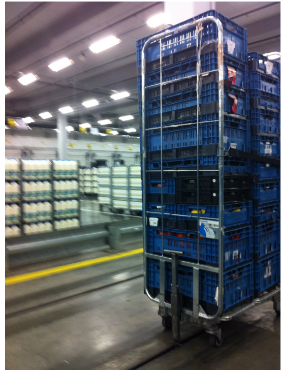
(b) Loaded carrier coupled onto the chain conveyor.
