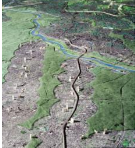
Figuur 24: Residential area should be concentrated within walkable circle of 800m diameter from railway stations. [Ohno 2006]
