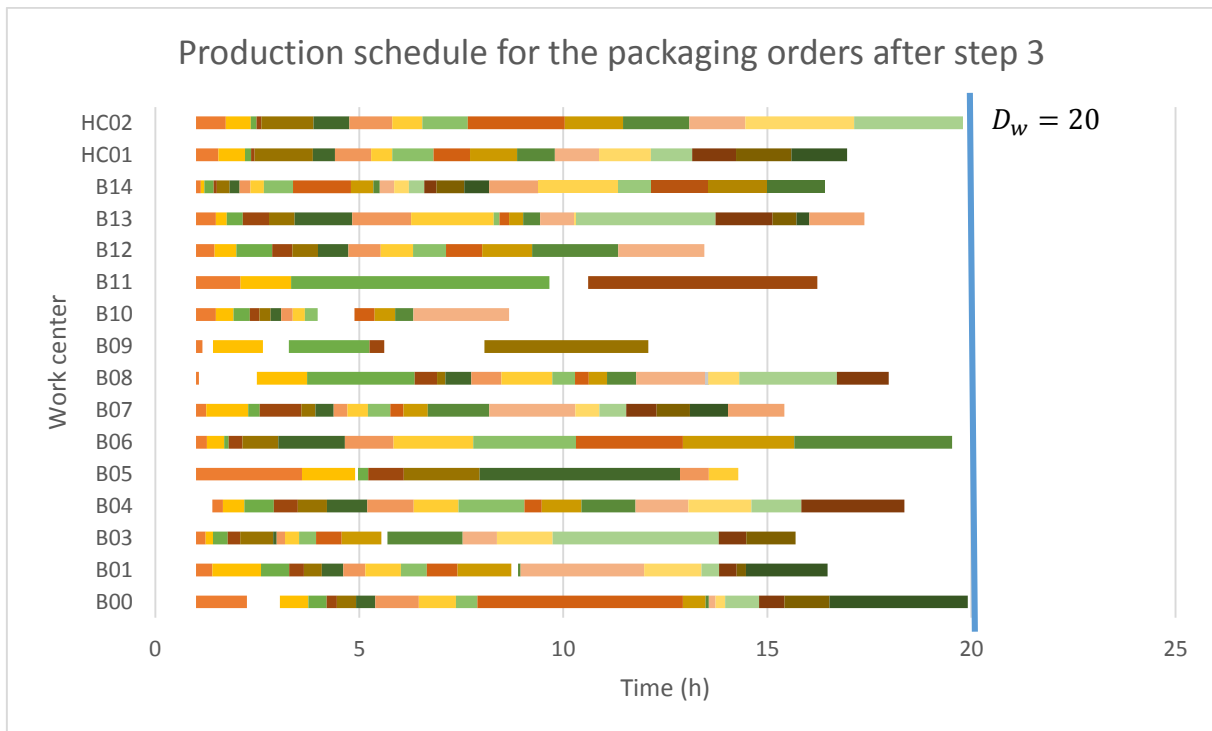
Figure 8.14: Production schedule for all packaging orders after step 3 of the solution approach
