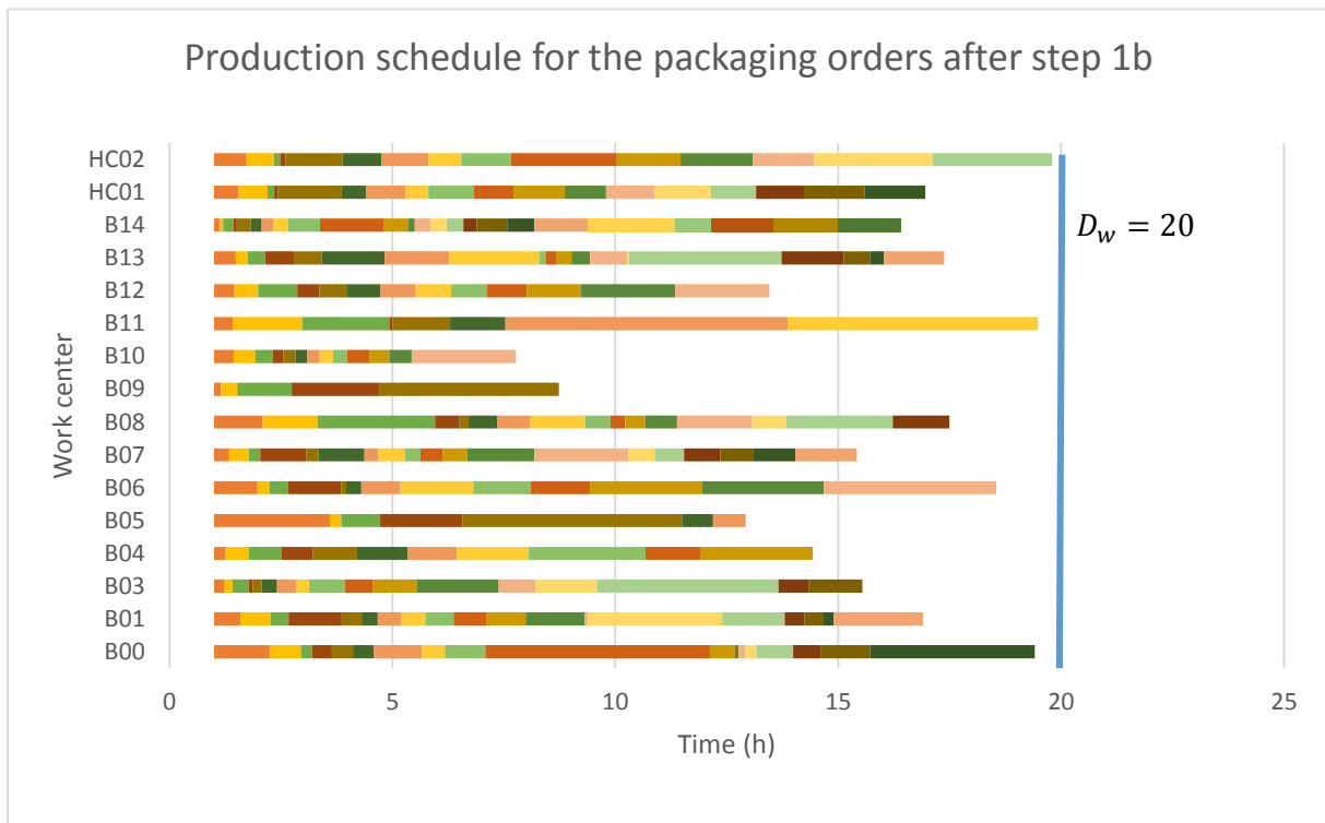
Figure 8.12: Production schedule for all packaging orders after step 1b of the solution approach.
