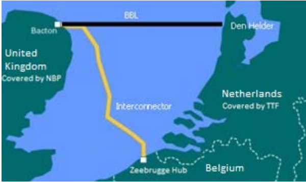
Figure 5. The pipelines connecting the NBP with the Zeebrugge hub and the TTF
