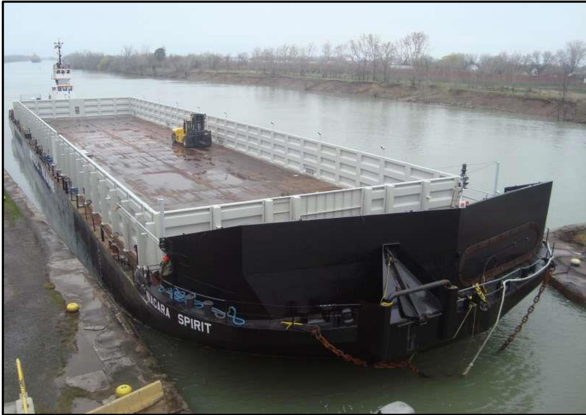
Figure 4.2: An example of a bin wall on McKeil's deck barge Niagara Spirit (McKeil, 2012).
