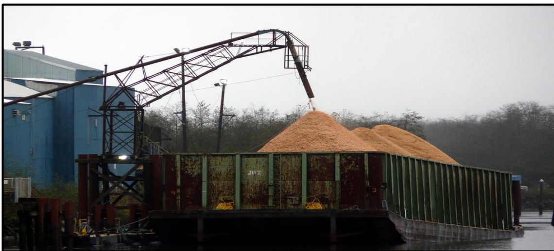
Figure 3.1: The loading of a woodchip barge via an automated system (Nsandal, 2012).
