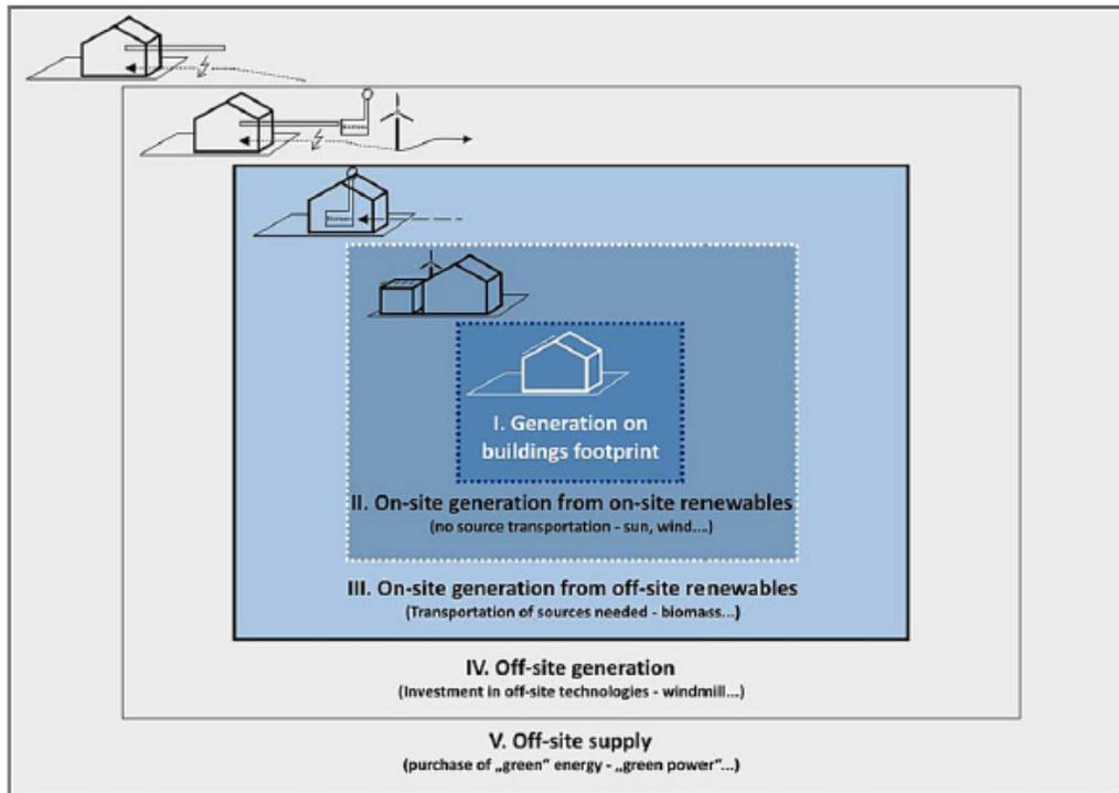
**Figure 1: Site configurations for residential ZNE. Source: (Marszal, Heiselberg, et al., 2011)**
