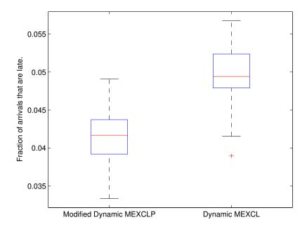
Figure 4: Fraction of arrivals that are late for Dynamic MEXCLP and MEXCLP respectively in a simulation with extra uncertainty in the driving times and with varying busy fractions.
