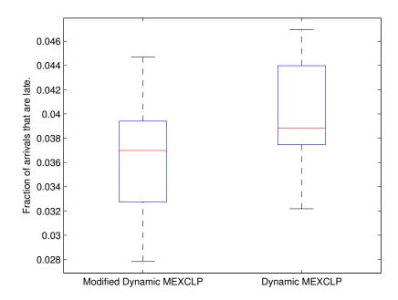
Figure 6: Fraction of arrivals that are late for Dynamic MEXCLP and MEXCLP respectively in a simulation with uncertainty in the driving times and with high varying busy fractions.
