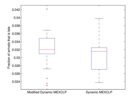
Figure 2: Fraction of arrivals that are late for Dynamic MEXCLP and the modified model respectively in a simulation without uncertainty in the driving times and without varying busy fractions.
