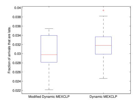
Figure 9: Fraction of arrivals that are late for Dynamic MEXCLP and the modified model respectively in a simulation without uncertainty in the driving times and with varying busy fractions.
