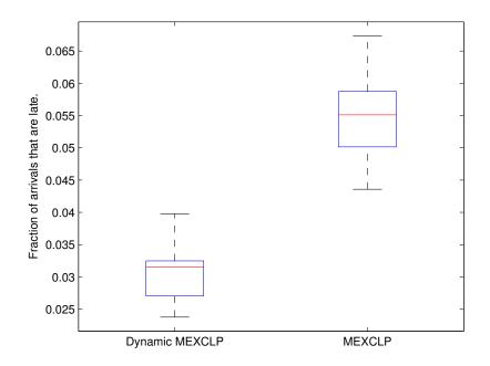
Figure 1: Fraction of arrivals that are late for Dynamic MEXCLP and MEXCLP respectively in a simulation without uncertainty in the driving times and without varying busy fractions.
