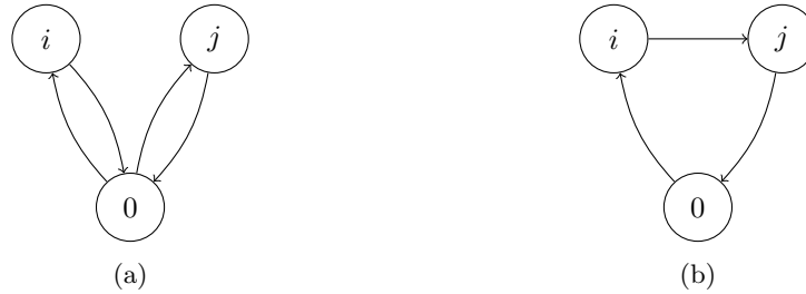
Figure 2: The saving algorithm. First, the customers i and j are in separate routes (a). These routes are connected by adding edge (i, j) (b).
