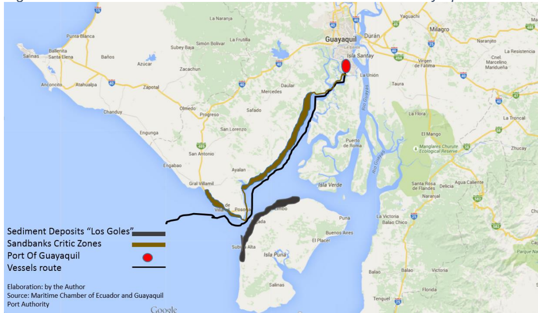
Figure 10 Actual situation of the Canal of Access to the Port of Guayaquil
