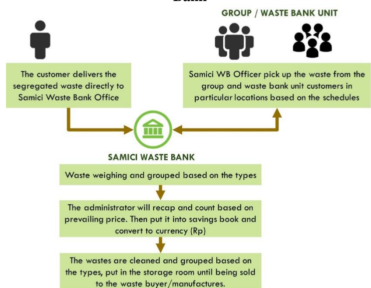
Figure 22 Flowchart of Waste Processing in Samici Waste Bank
