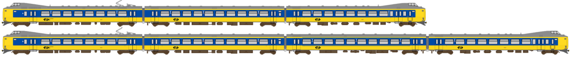
Figure 2.1: Two train units of the same type: ICM, but different subtypes: ICM3 and ICM4.
