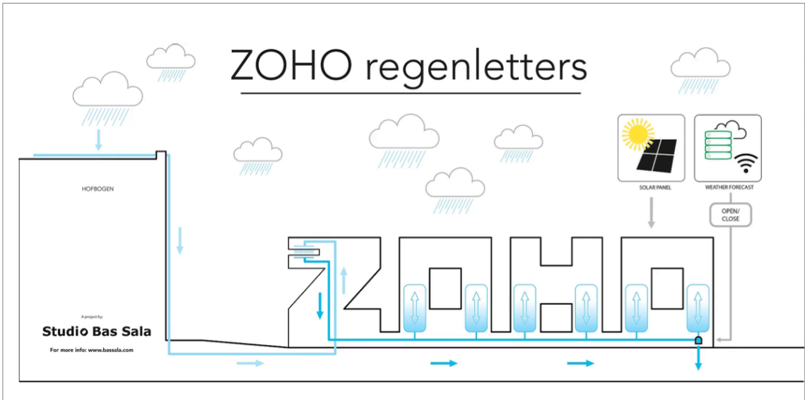
Figure 34 Water system in the ZOH O letters by Studio Bas Sala ( source: Studio Bas Sala, 2019)
