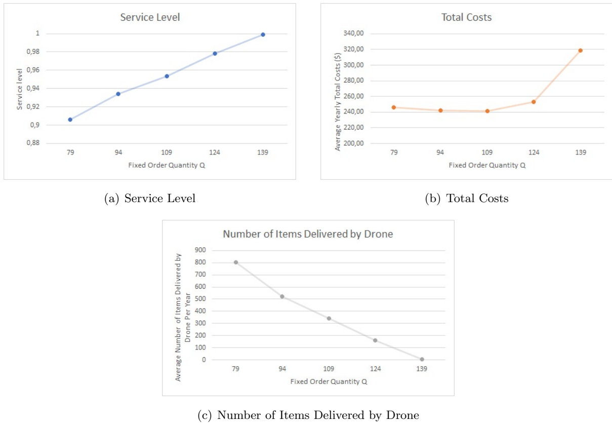
Figure 9: Model Performance for Different Values of Fixed Order Quantity Q and a Targeted Service Level of 95 %
