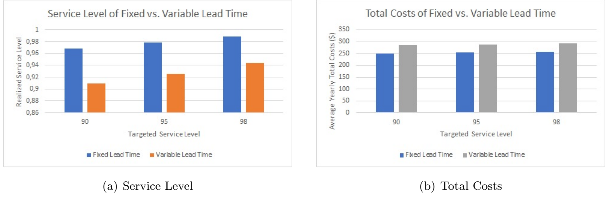
Figure 11: Model Performance under Fixed and Variable Lead Time for Different Targeted Service Levels
