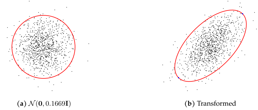
Figure 4.15. 1000 random sampled points and the 95% confidence interval (CI). The set of points is transformed (right), such that the CI represents an ellipse with major axis endpoints intersecting the waypoints in blue, and minor axis scale factor c_{\text{insert}} = 0.5 .
