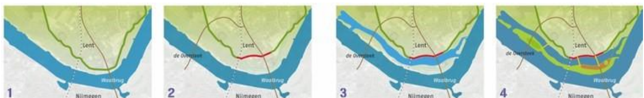
Figure 2-4: 1) the current situation with the existing dike 2) relocation of the dike 350 inland 3) digging a secondary channel giving the river more room, which created an island 4) connecting the channel banks with bridges.
