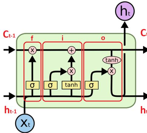
Figure 4.2: LSTM cell architecture
