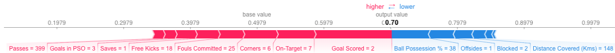
Figure 8: Example that illustrates the process of SHAP values where the predicted value, equal to 0.498, is obtained from the base value, equal to 0.700, by adding the contributions of all the different features to the base value.
