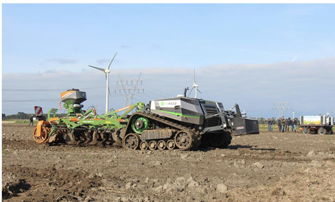
Figure 10 – AgXeed AgBot Tracked tractor equipped with a cultivator and a visual yield measurement system. (NPPL, 2021)
