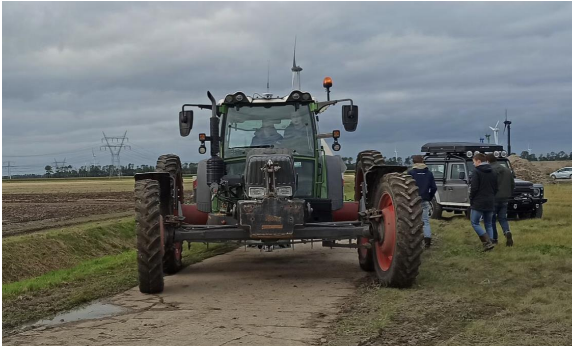
Figure 7 – Tractor with adjusted width of the axis (Author, 2021)
