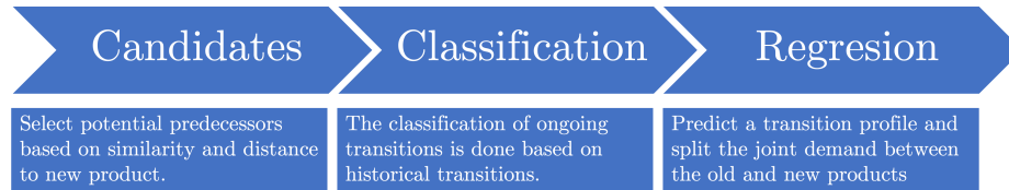
Figure 10: Three staged prediction approach
