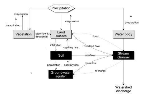
Figure 4 System concept of the runoff process. Source: (Feldman, 2000, p10)
