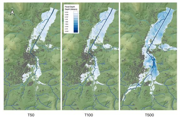
Figure 30 Flood maps for the scenario 2021, for different return periods.
