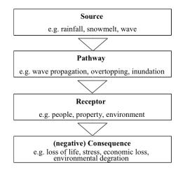
Figure 2 Source-Pathway-Receptor-Consequence Concept. Source: (Schanze 2009, p 4)
