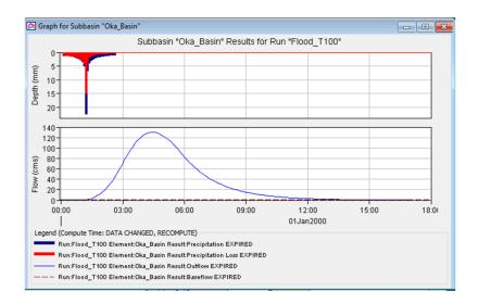
Figure 25 HEC-HMS Oka river model results T100, 2021 Scenario.
