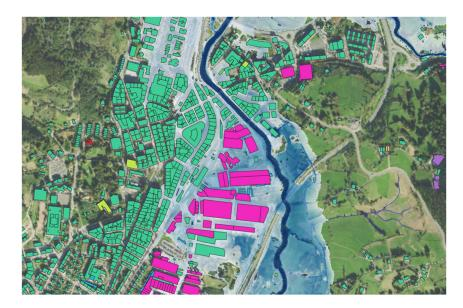
Figure 32 Detail of the flood map for the 2021 scenario and 500 years return period.
