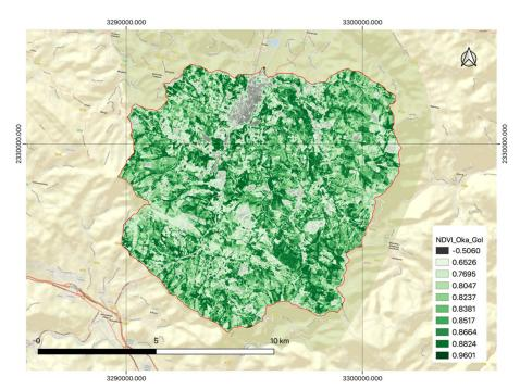
Figure 16 Normalized Difference Vegetation Index (NDVI), Sentinel-2A, June 6 2021. Bands Combination (B8-B4/B8+B4).
