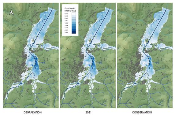
Figure 33 Flood maps for the degradation, 2021 and conservation scenario, for a return period of 500 years.
