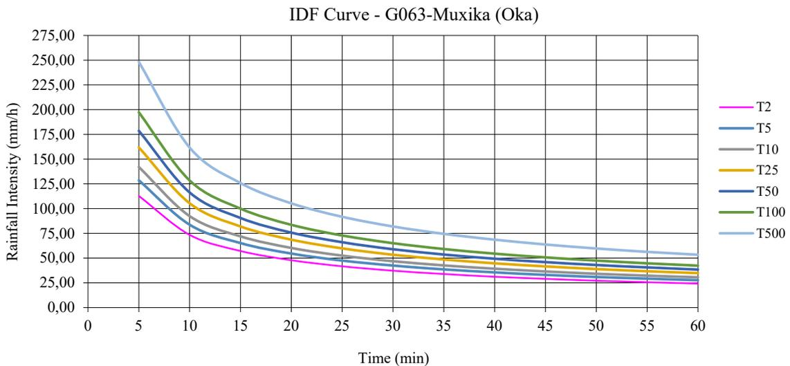
**Figure 9 Intensity-Duration-Frequency Curve G063 – Muxika (Oka)**
