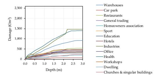
Figure 36 Flood Depth Damage Curve for Gernika-Lumo (Martinez-Gomariz et al, 2020)
