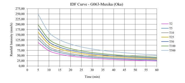
Figure 9 Intensity-Duration-Frequency Curve G063 – Muxika (Oka)
