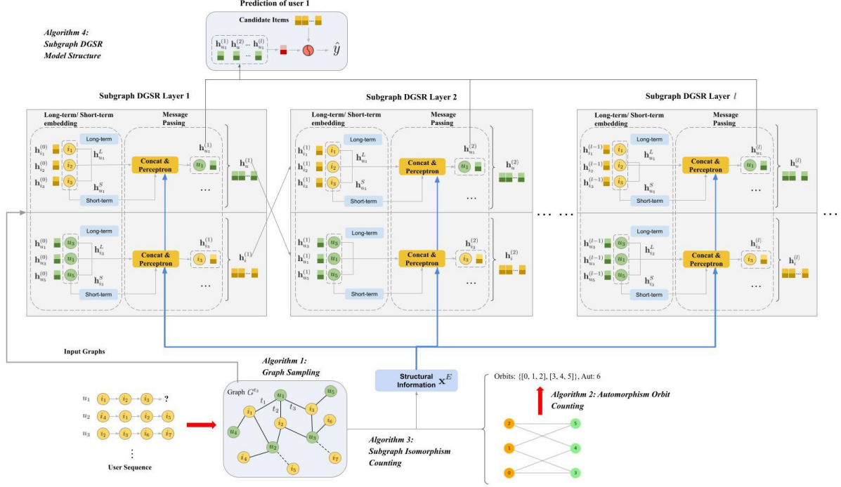
Fig. 1: The overview of Subgraph DGSR framework, taking the prediction of u_1 with interaction sequence (i_1, i_2, i_3) as an example. Starting at the bottom left corner, we convert users' interaction sequences into dynamic graphs G_{t_3} , and perform Algorithm 1 and get a m -order sample graph G_{u_1}^m(t_3) (Section 4.1). Before imputed to the model, we perform Algorithm 3 (Section 4.2.2) to generate structural information from G_{u_1}^m(t_3) with orbits of the subgraph list. The orbits are counted by Algorithm2 (Section 4.2.1) when the model is set up. After this, the well-designed Subgraph DGSR model (Algorithm 4; Section 4.3) will propagate and aggregate the information and finally output the prediction
