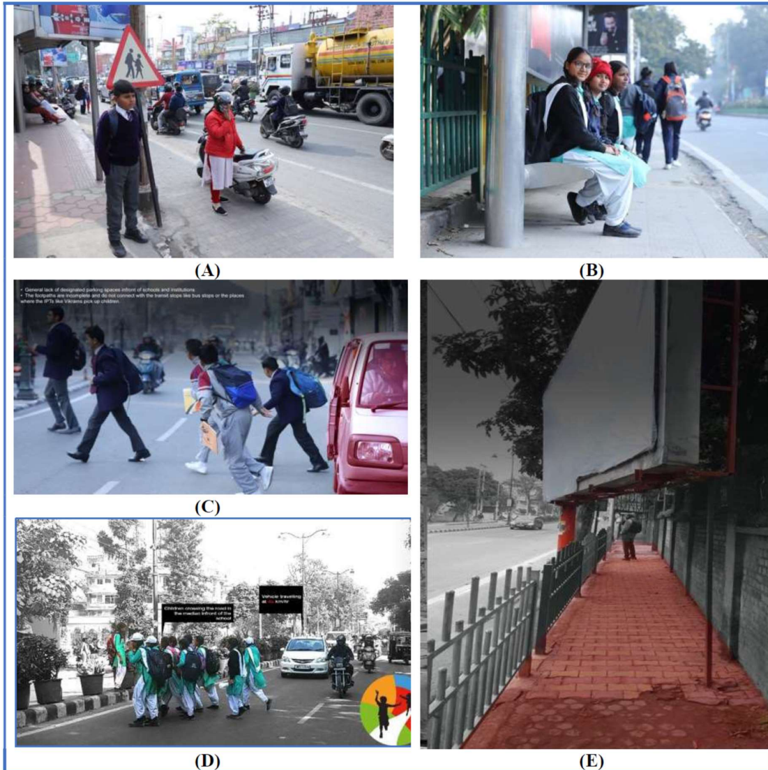
(A) Demarcated road crossing without zebra crossing, (B) Bus stop without dedicated lane, (C) and (D) students crossing road amidst of running traffic showing the threat, and (E) Footpath blocked by the commercial signage making it inaccessible. (Courtesy: Dehradun Smart City, Personal Communication).
