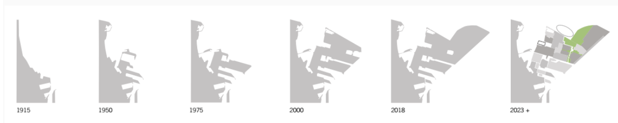
Figure 5.13. The growth of Nordhavn through landfill. From Structure Plan Ydre Nordhavn, 2023 revision (By & Havn, Cobe, Sleth, & Raw Mobility, 2023, p. 62)
